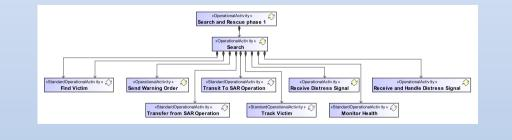
The **Operational Process Flow (Op-Pr)** diagram depicts a workflow, showing processes and information passing between processes. The diagram utilizes SysML Activity Diagram notation to model Control Flow and Object Flow between Operational Activities, including decision and merge, as well as fork and join logical operators.
